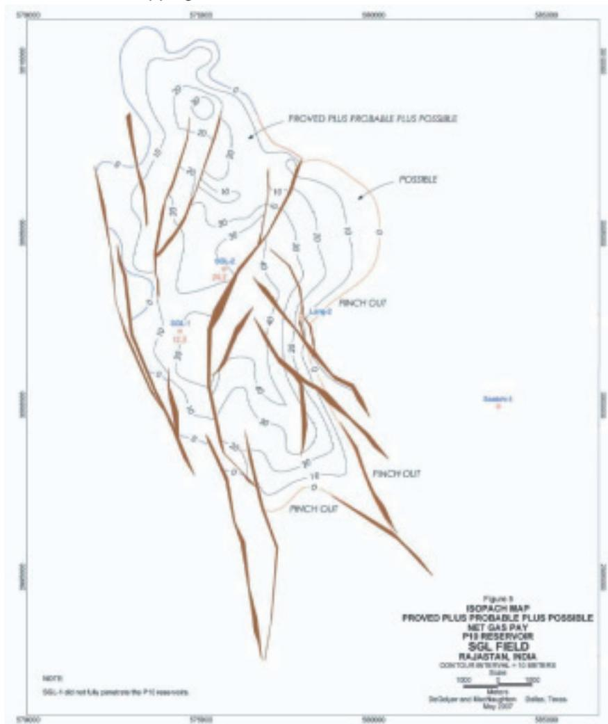
**Figure 4-1** Isopach map showing 2P and 3P net pay thickness (source D&M)
